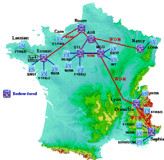
Figure 10.4: High speed network (2.5Gb/s) between INRIA research centers and several other research institutes.
